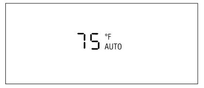
When in AUTOMATIC and weather conditions require heat, air will be sent to the floor. However, a feature is included in your EATC to prevent blowing cold air to the floor if the engine coolant is not warm enough to allow heating. In 3 1/2 minutes or less, the fan speed will start to increase and the air flow will be to the floor area.
